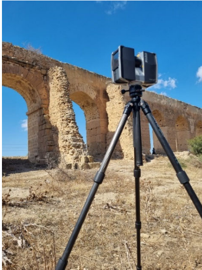
Fig. 1: Building survey using 3D laser scanning at the aqueduct in the Miliane Valley (I. Mayer, ÖAW-ÖAI 2021)
