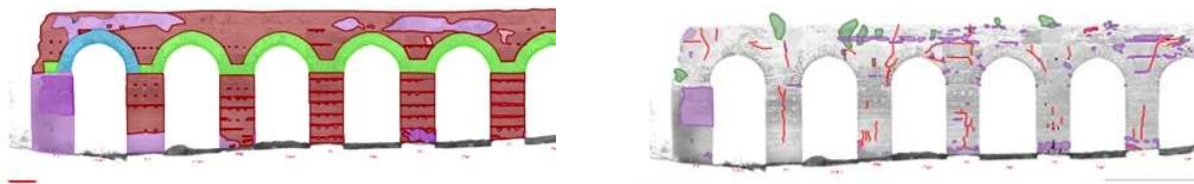
Fig. 4: Digitization of the inventory and condition mapping carried out on the aqueduct section in the Miliane valley
