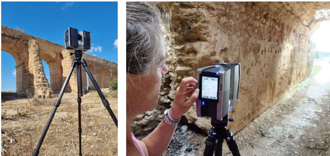
Fig. 7a, b: 3D laser scanning of the aqueduct in the Miliane valley (I. Mayer, OeaW-OeAI Wien 2021)
