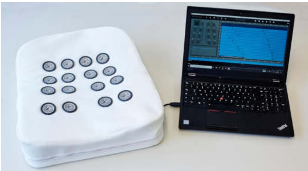
Multi-channel lung sound recording device (developed at TU Graz). © SPSC, TU Graz
